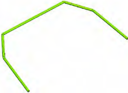
Image shows CAD data of front stabilizer.
