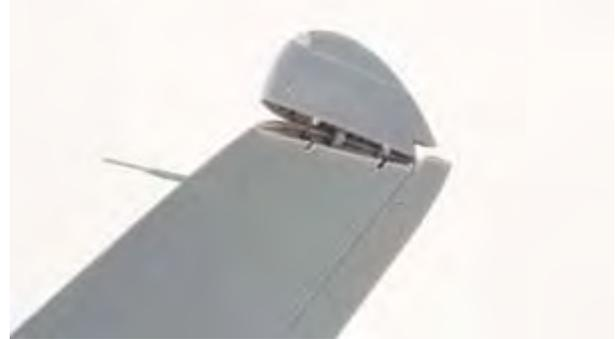
Photo-etched parts allow the wingtips to be set in the folded position.
