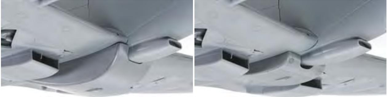
Image shows the 90 gallon (left) and 30 gallon (right) fuel drop tanks.
