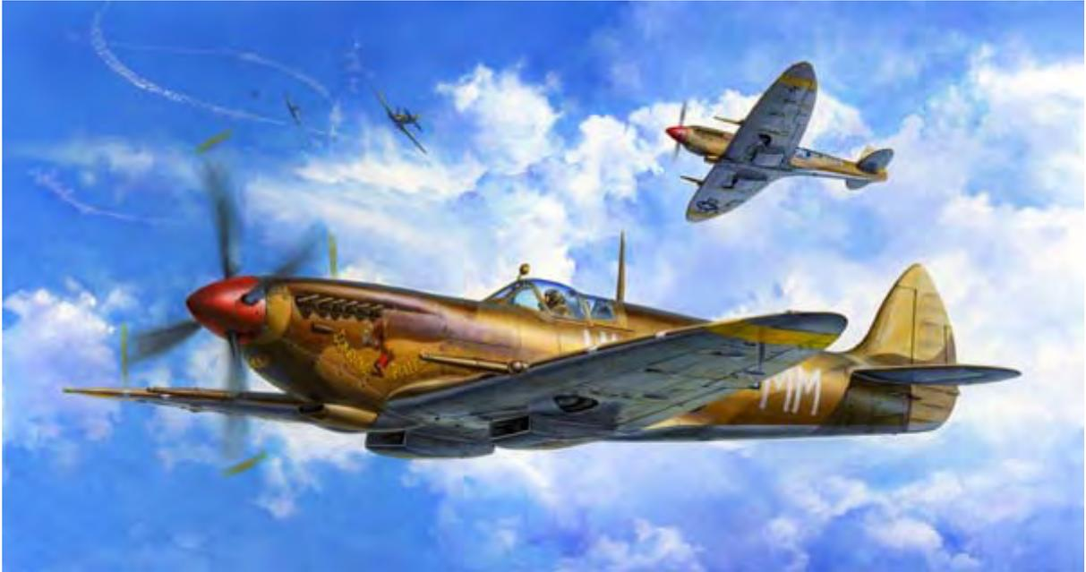
The Spitfire Mk.VIII was developed to succeed the Mk.V and was powered by a Merlin 60 engine. It also included many new improvements such as an enlarged rudder, shortened ailerons, a retractable tail landing gear, and fuel tanks installed at the leading edges of the wings. The Mk.VIII finally went into service in the summer of 1943, after the deployment of the stop-gap Mk.IX.
