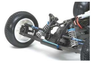
Aeration dampers feature new coil springs. Suspension has been designed to achieve excellent handling performance. Front axles are compatible with wheels using metric size ball bearings (For information on front axles for wheels using inch size ball bearings, refer to Item 54220 on page 37).
