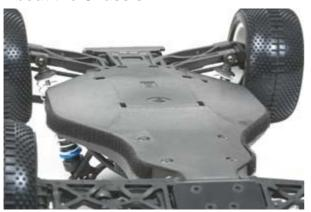
Chassis frame is made from fiberglass reinforced nylon resin and features a longitudinal battery position. Rear section is designed for optimized chassis roll balance. Chassis shaped is designed for an improved center of gravity whilst providing sufficient ground clearance.
