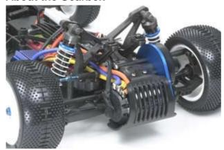
Gearbox is equipped with a ball differential which features inch sized diff. balls (12pcs.), 2.6mm dia. diff screw, and newly designed thrust ball bearings. Diff. carrier features a new teeth shape to ensure a long-lasting performance. Suspension is fitted with assembly universal shafts.
