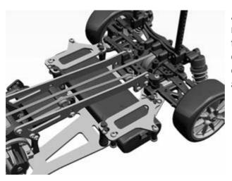
Adjustable battery holder enables attachment of Tamiya Ni-Cd, Ni-MH, and LF battery packs (battery packs can also be secured with glass tape). R/C units are placed centrally on the chassis for optimized balance.
