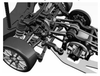
Features TA05 bulkheads, short reversible suspension arms, TRF416 uprights. 37T front and rear pulleys and 18T center pulley are driven by new-length drive belts. Belt tensioner is also equipped.
